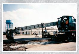
for the high productivity removal of the old asphalt and ties. The delicate boom functions, requiring less power and less fuel consumption, complete the placement of the new asphalt between the rails, and smooth the material outside the rails. As a result, the Model XL 3300 saves money on the cost of bringing additional machines to the site, and for labor since there's not much need for hand work in spreading asphalt. Tim Wilson, the city's director
