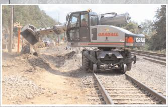
alongside the tracks. \* "This machine does everything," said Hoffer, a Gradall machine operator for the railroad for the past three years. In fact, Norfolk Southern also uses the Gradall machines to build and repair right-of-ways, clear vegetation and replace rails. \* For information, contact Gradall at 330-339-2211.
