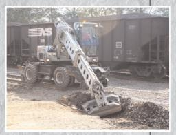
machine can travel around 22 mph on rails, and it did not need the highway to be re-opened to access the tracks. In fact, the Gradall machine was able to re-open the tracks for train travel long before automotive traffic was restored on the adjacent highway. Using an excavating bucket and a ditching bucket, and the well-known Gradall tilting, telescoping boom movement, operator George Hoffer Jr. was able to clear dirt and rocks from between the rails as well as
